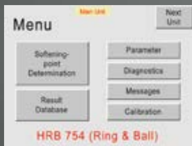
A. The HRB 754's "touch screen" display lets you quickly initiate standard softening point tests, change test parameters, run system diagnostics, and recall test results.
